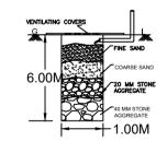
RAIN WATER HARVESTING STUCTURE DETAILS
